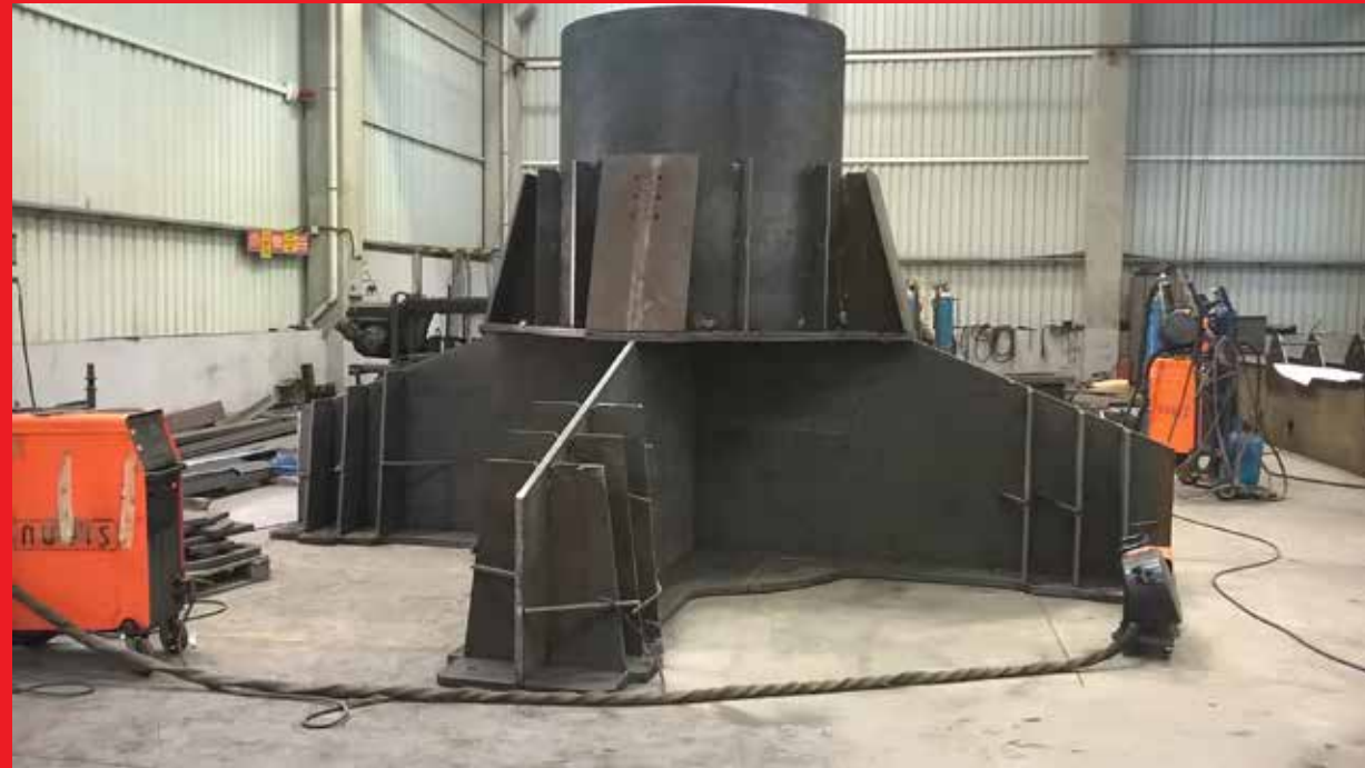
Port Tower Crane Base
